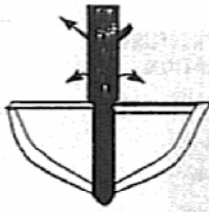
Mixing tool for constructing Lime Cement Columns™.
